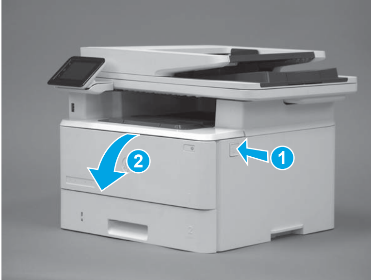
Figure 1-2 Open the toner-cartridge door
