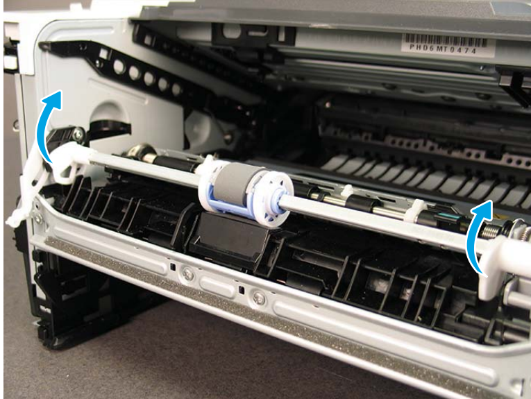
Figure 1-1038 Rotate the Tray 1 pickup roller shaft
