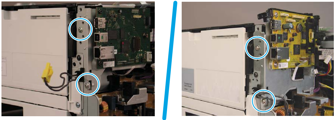
Figure 1-574 Remove two screws
