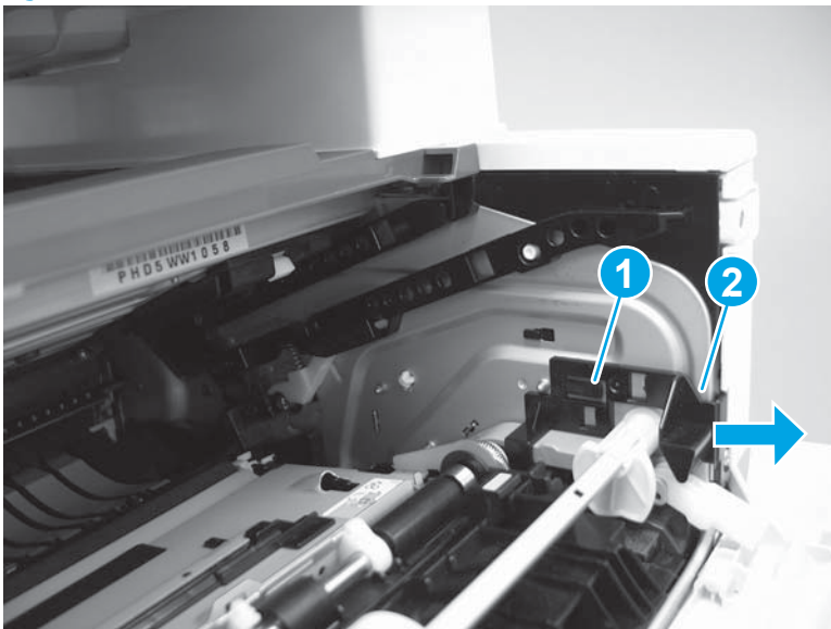
Figure 1-420 Remove the guide
