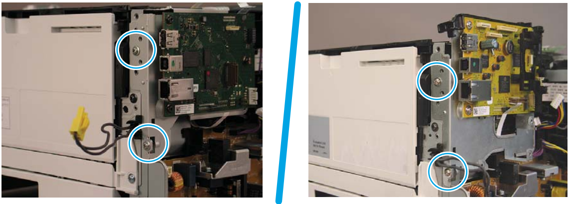
Figure 1-640 Remove two screws
