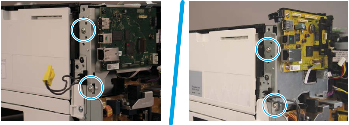
Figure 1-897 Remove two screws
