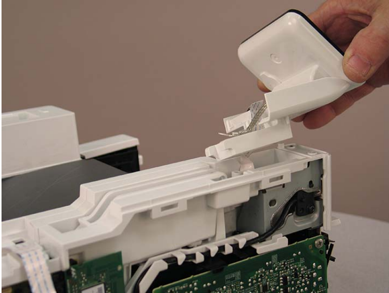
Figure 1-627 Lift up the control-panel assembly
