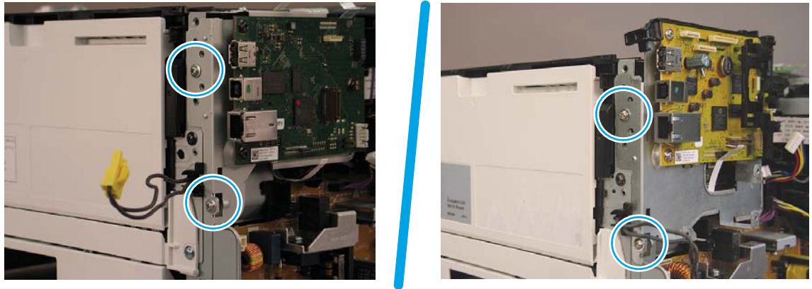
Figure 1-742 Remove two screws
