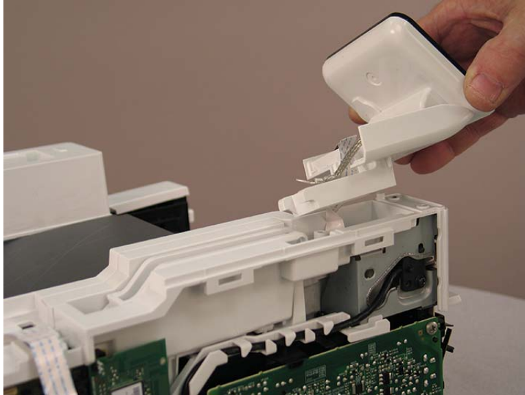
Figure 1-677 Lift up the control-panel assembly
